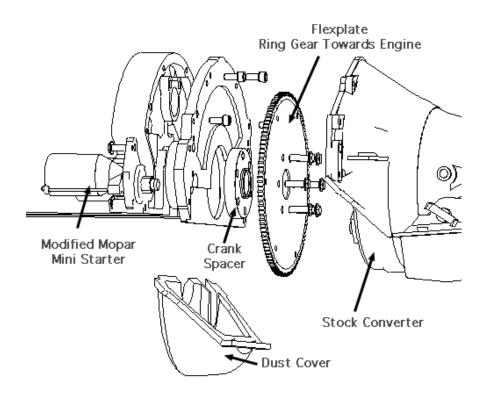
CLEAN THE CRANKSHAFT FLANGE AND HUB USING SOLVENT AND A RAG AND INSPECT FOR BURRS, DINGS, NICKS, ETC. THIS IS CRITICAL! THE ALIGNMENT OF THE ENTIRE ROTATING ASSEMBLY RELIES ON THE FACE OF THE CRANKSHAFT AND THE HUB SPACER MATING EXACTLY. REMOVE ANY BURRS WITH A FINE PITCH FILE.
