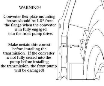
PLEASE NOTE; WHILE INSTALLING THE TRANSMISSION, REMEMBER THAT THE DOWEL PINS ARE FOR ALIGNMENT ONLY AND WILL NOT BEAR THE WEIGHT OF THE TRANSMISSION. CHECK THAT THE CONVERTER IS SEATED INTO THE FRONT PUMP PRIOR TO INSTALLING THE TRANSMISSION.
