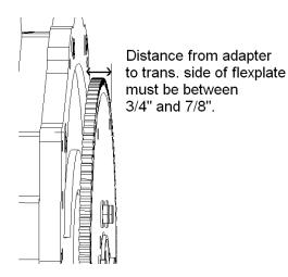
CHECK THE DISTANCE BETWEEN THE TRANSMISSION SIDE OF THE FLEXPLATE AND THE ADAPTER. THIS SHOULD BE BETWEEN .750" AND .875". **DO NOT PROCEED WITH THE INSTALLATION IF THIS IS NOT CORRECT.** ASSEMBLING THE MOTOR TO THE TRANSMISSION WITH THIS DIMENSION NOT IN TOLERANCE COULD RESULT IN TRANSMISSION OR STARTER DAMAGE. CONTACT WILCAP IF YOU FIND THIS DIMENSION TO BE GREATER THAN 7/8" OR LESS THAN <sup>3</sup>/4".
