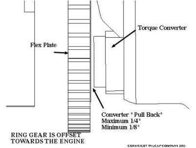
ALIGN THE CONVERTER AND THE FLEXPLATE HOLES AND START EACH BOLT. ROTATE THE ENGINE AS YOU TORQUE THE CONVERTER BOLTS TO THEIR FINAL VALUE IN AT LEAST THREE STEPS.
