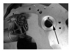
REMOVE THE ADAPTER PLATE AND MARK STRAIGHT OUT TO THE EDGE OF THE BELLHOUSING FROM THE EDGES OF THE CIRCLE.
